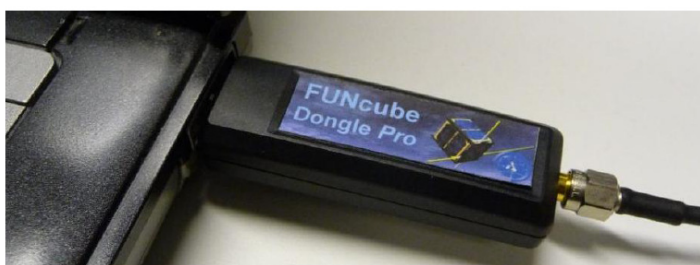
Figure 3. The Original FunCube Dongle Pro SDR
