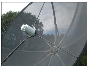
3m Dish with 1420MHz Feed
