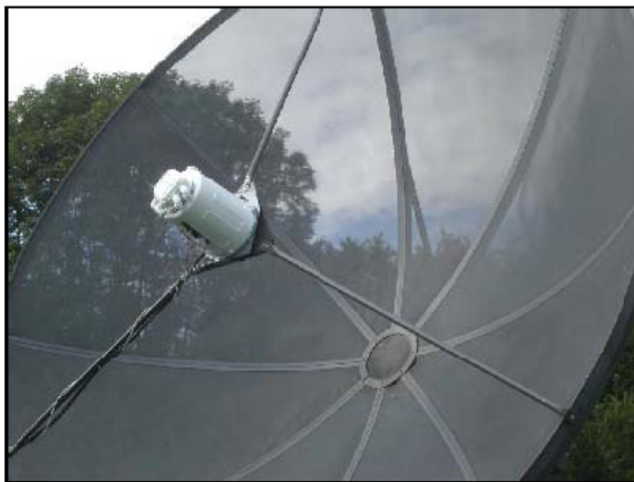
Figure 1. 3m focal plane dish and 1420MHz feed
